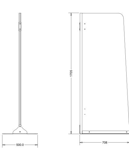
The Hygiene Screen is a combination of aluminium frame & 3mm steel base with an acrylic panel to provide peace of mind and a safe barrier between clients.
